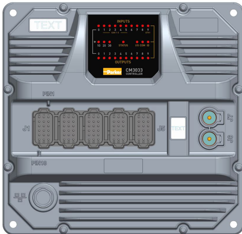
Figure 4: IQAN-Open CM3033 connector configuration
